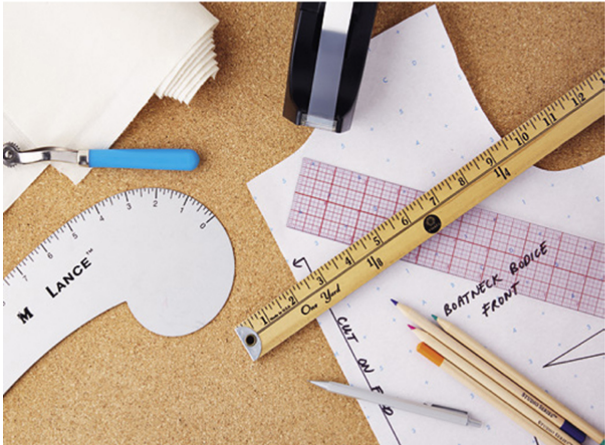
SUPPLIES FOR PATTERN TRACING (clockwise from upper left): muslin, tape, yardstick, clear ruler, colored pencils, mechanical pencil, French curve, tracing wheel, corkboard
